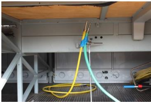
Ir-192 gamma source in baggage compartment of bus (1.5 TBq)
