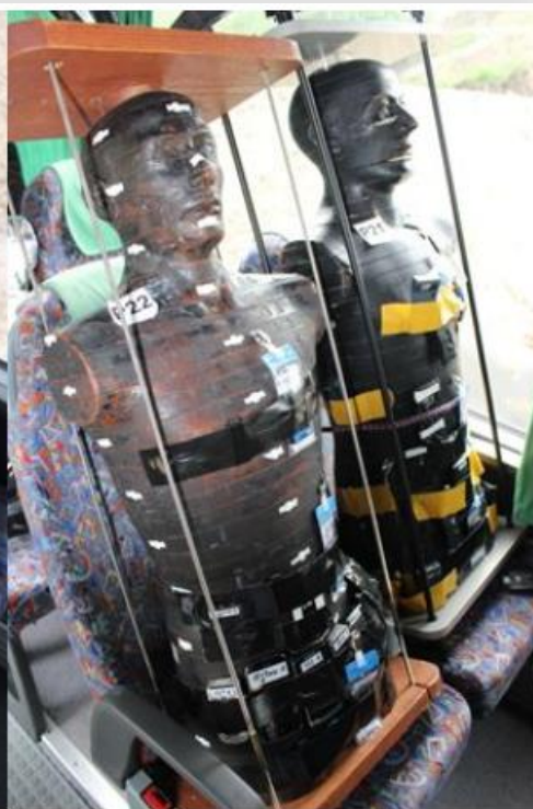
Water-filled canisters and anthropomorphic phantoms with attached mobile phones and reference dosimeters (EPDs, OSLDs and TLDs)
